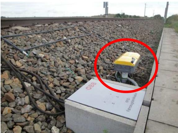
Figure 8: Typical “Rail-Reader” field installation
