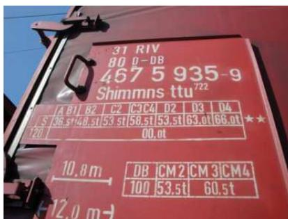
Figure 2: Technical parameters describing a wagon
