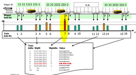
Figure 5: “Rail-Reader” allocate numbering of the “wagon axles”
