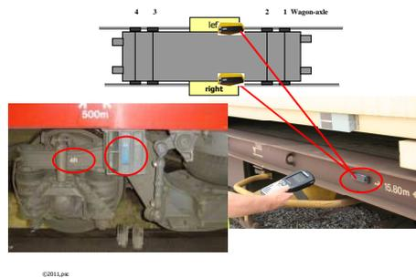
Figure 3: “Numbered” wagon-axle
