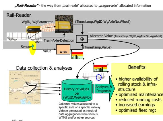
Figure 1: From “train-axle” allocated to “wagon-axle” allocated information
