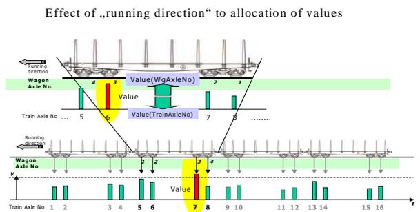
Figure 6: Handling different situations of running direction
