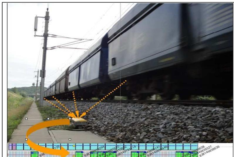
Figure 1 – example of an RFID AVI system used in railway transport
